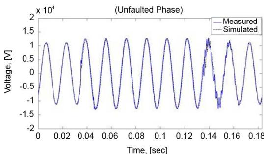
Fig. 14. Phase C (unfaulted phase) voltage at the secondary terminals of the area substation transformer.
