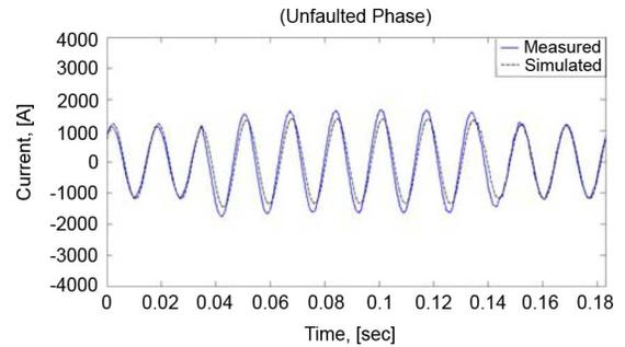
Fig. 16. Phase B (unfaulted phase) current at the secondary terminals of the area substation transformer.
