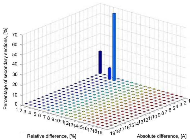
Fig. 10. Comparison of secondary currents of a large-size network calculated using the commercial PF program and EMTP time-domain simulator.
