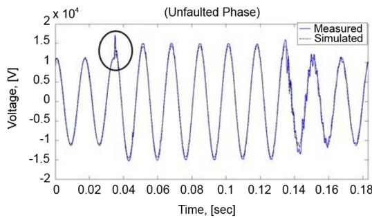
Fig. 13. Phase B (unfaulted phase) voltage at the secondary terminals of the area substation transformer.
