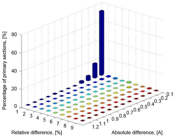
Fig. 5. Comparison of primary currents in a small-size network calculated using the commercial PF program and EMT-P time-domain simulator.
