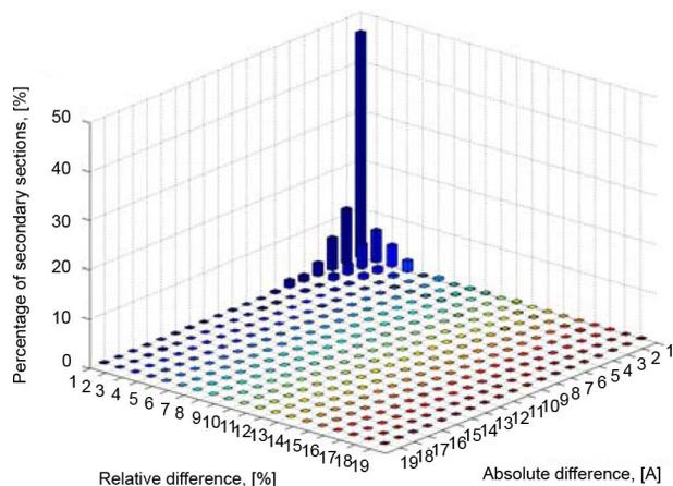
Fig. 9. Comparison of secondary currents in a middle-size network calculated using the commercial PF program and EMTP time-domain simulator.
