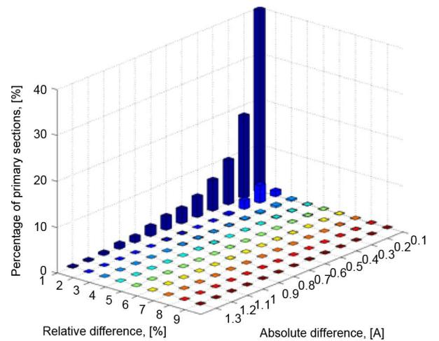
Fig. 7. Comparison of primary currents of a large-size network calculated using the commercial PF program and EMT-P time-domain simulator.
