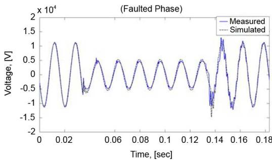
Fig. 12. Phase A (faulted phase) voltage at the secondary terminals of the area substation transformer.
