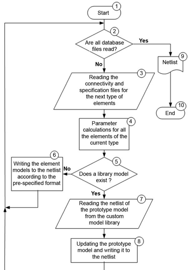
Fig. 1. Flowchart of the data translation from a power-flow database to EMTP.
