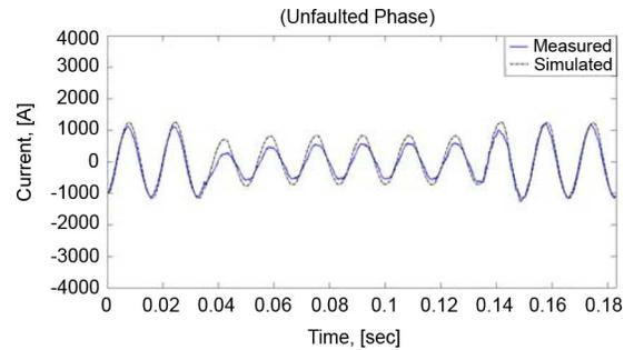
Fig. 17. Phase C (unfaulted phase) current at the secondary terminals of the area substation transformer.
