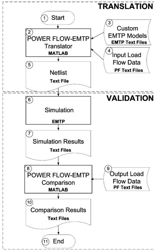
Fig. 4. Block diagram of the POWER FLOW-EMTP translator.
