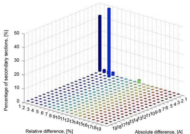
Fig. 8. Comparison of secondary currents in a small-size network calculated using the commercial PF flow program and EMT-P time-domain simulator.
