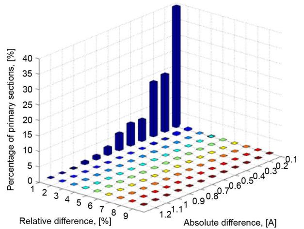
Fig. 6. Comparison of primary currents in a middle-size network calculated using the commercial PF program and EMT-P time-domain simulator.
