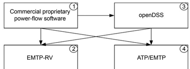
Fig. 2. Scheme of a one-way power-flow data translation.
