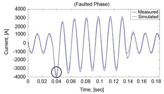
Fig. 15. Phase A (faulted phase) current at the secondary terminals of the area substation transformer.
