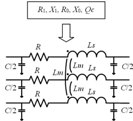
Fig. 3. Example of the conversion of a transmission-line section from the power-flow databases into the EMTP netlist.
